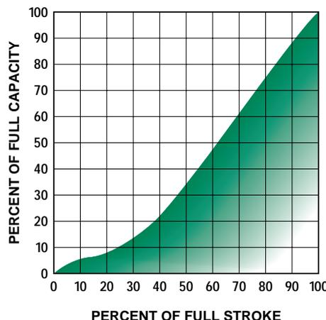
**Figure 19-1.** Parabolic Plug Metering Valve
