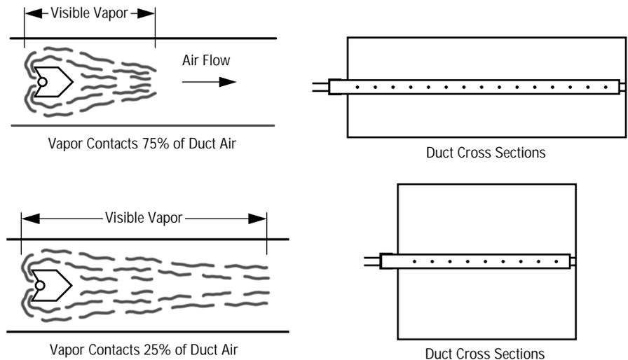
**2. Duct Air Temperature.** The temperature of the air flow in the duct also affects the length of the visible vapor pattern. Warmer air produces shorter vapor pattern, as shown in Fig. 23-1. All other conditions are the same. In 75°F duct air, the average vapor output from a manifold produces a visible vapor pattern shorter than 12 inches in length.
