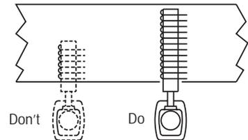
The manifold should never be installed vertically downward from the humidifier. This presents a condensate drainage problem in the jacket of the manifold. Vertical upward installation is permissible.
