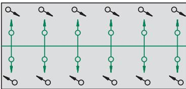
**Figure 37-2.** Outlines a typical requirement. Schematic layout of humidifiers in wood-working plant where exhaust fans are used. Arrows indicate air flow induced by fans. Humidifiers are sized for load conditions imposed by fan. Humidifiers are located to give uniform distribution of humidity when fans are off or when fans are running.
