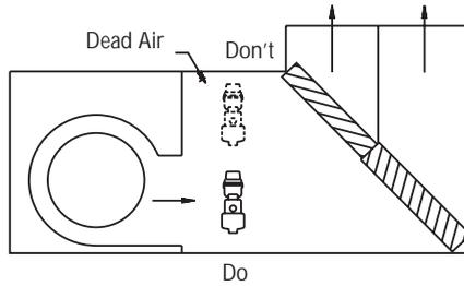
Do not install a distribution manifold closer than 10 feet upstream from a temperature controller or you may get false signals.
