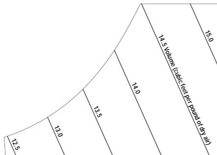
**6. Volume lines** indicating cubic feet per pound of dry air are plotted at intervals of .5 cubic foot.
