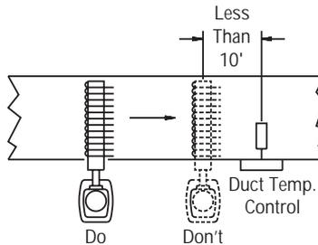
The distribution manifold should never be placed within three feet of an air fan intake. The best location is at the fan discharge.
