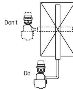
Always select the stream distribution manifold length that will span the maximum width of the duct.
