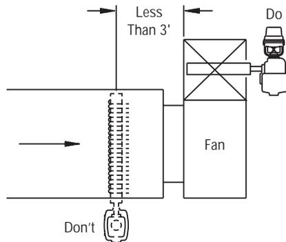
Whenever possible, install the distribution manifold into the center of the duct.
