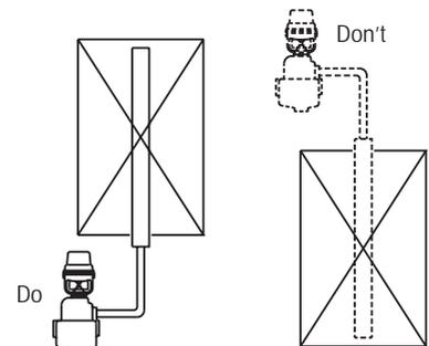
NOTE: All dimensions shown in the above figures are based on duct temperature of 65°F or higher and duct velocities of 800 ft/min, or lower. If duct air is cooler or velocities are higher, these dimensions should be greater or multiple manifolds considered.
