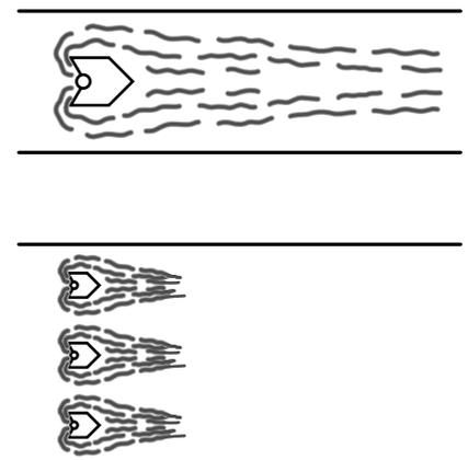
Since the use of multiple manifolds reduces the length of visible vapor, their use should be considered whenever any of the following conditions exist at the humidifier location:
