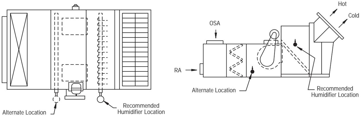
Figure 34-2. High Pressure System
