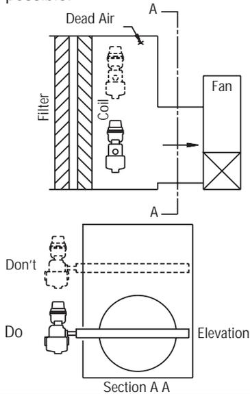
Don't risk restriction of the air flow in ducts 8" or less in depth. Use an expanded section as shown.
