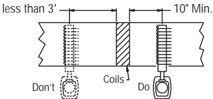
When it is necessary to place the humidifier in the coil section ahead of the fan, locate the manifold in the most active air flow and as far upstream from the fan inlet as possible.
