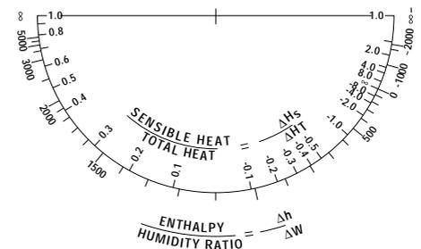
**8. The protractor** at the upper left of the chart contains two scales. One is for the ratio of enthalpy difference. The other is for a ratio of sensible heat to the total heat. The protractor establishes the angle of a line on the chart along which a process will follow.
