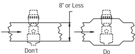
When it is necessary to place the humidifier discharge into a packaged multi-zone air handling system, install the distribution manifold into the center of the active air flow and as close to the fan discharge as possible.
