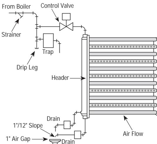
NOTE: Condensate cannot be lifted or discharged into pressurized return.
