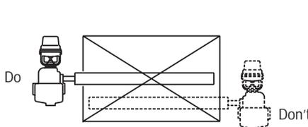
Always install distribution manifolds as far upstream from discharge air grilles as possible—never less than three feet upstream.
