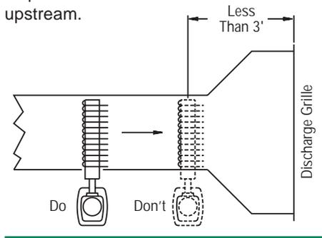
Always size and install the distribution manifold to span the widest dimension of the duct section.
