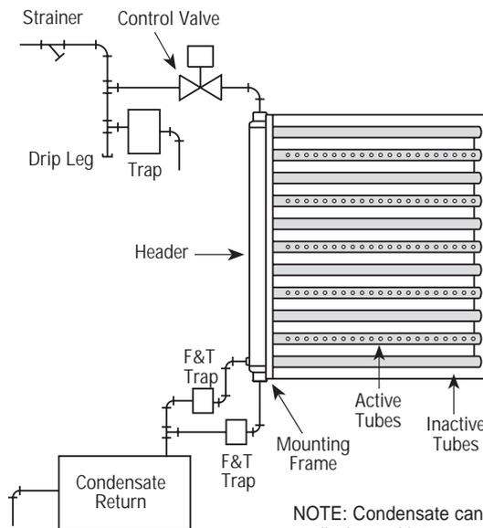
NOTE: Condensate cannot be lifted or discharged into pressurized return.
