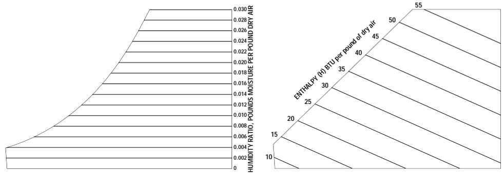
**1. Humidity ratio values** are plotted vertically along the right-hand margin, beginning with 0 at the bottom and extending to .03 at the top.
