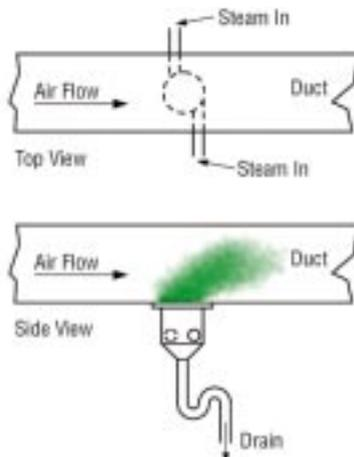
Figure 18-3. Steam Separator Type Humidifier
